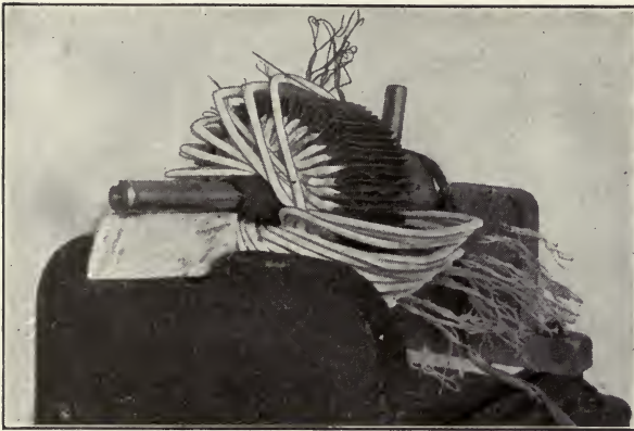
FIG. 67.—All bottom sides of coils in place and strips of insulation inserted between bottom and top coil sides ready for the top layer of the winding.
